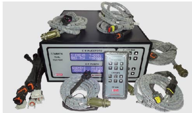
CRT 7000 - Common Rail Injector, Pump & Rail Tester (with computer interface/software) (Euro IV & V Compliant)
