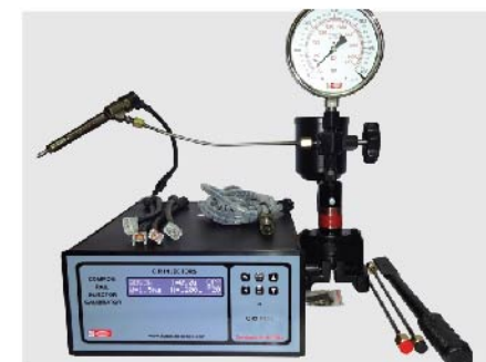
CRIH 4100 - Common Rail Injector Testing Hand Operated Kit
