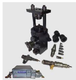
Cam Box for EUI & EUP with Simulator
